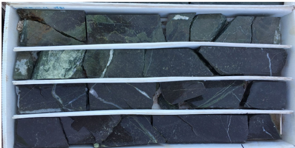
Figure 7-16 Weakly veined and sulfidic andesite, 110.90m to 112.05m, SCGP-26, which assayed 294 gpt Ag, 0.006 gpt Au, 0.2% Pb, 0.1% Zn, and 0.01% Cu
