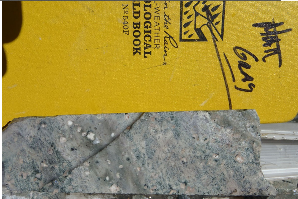
Figure 7-10 ¼ HQ core of banded rhyolite dike, adjacent to mineralized breccia, 54.5m depth, drillhole SCHN-01. This dike assayed 7 gpt Ag and 0.2 Pb and 0.3% Zn.
