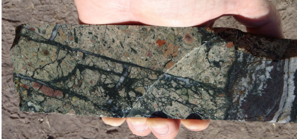
Figure 7-17 Brecciated lithic andesite tuff with siliceous-chloritic-sulfidic matrix crosscut by banded quartz-sulfide veinlet (right extreme of core sample), drillhole SCHN-08, 87.7m. The breccia crosscut by the vein in the interval 86.95 to 97.70m assayed 876 gpt Ag, 0.022 gpt Au, 0.2% Pb, 0.1% Zn, and 0.03% Cu. The breccia on either side of this interval without quartz-sulfide veining assayed 30 gpt Ag.
