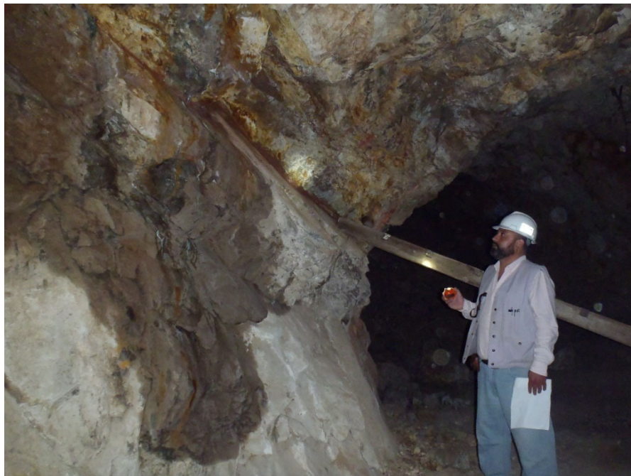
Figure 7-20 Santacruz Silver geologist Miguel Angel Torres in San Marcial working on the Guadalupe mineralized structure. Planar fault boundary forms the footwall to the mineralized zone (wooden ladder rests on the footwall structure).
