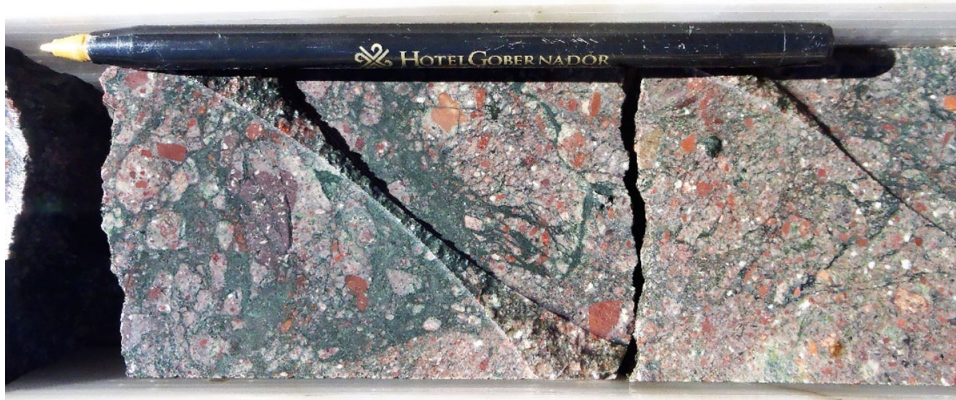
Figure 7-14 Detail of 1/2 HQ core of mineralized multi-stage breccia, drillhole SCHN04, 114.80 to 115.85m. Although not readily visible in photo, breccia matrix contains several percent disseminated dark sulfide, presumably acanthite.
